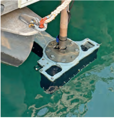
The sonar system, an R2Sonic 2026V capable of scanning a swath of up to 1,024 beams, is mounted on the Dr. Robert Werner Research and Education Boat, provided by the Skaneateles Lake Association for the survey.
